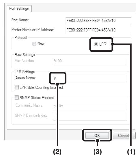
**(1)** Select [LPR].**(2)** Enter [lp].**(3)** Click the [OK] button.**7** Click the [Next] button in the screen of step 5.**8** Click the [Finish] button.**9** Click the [Close] button in the screen of step 2.**When using a port created with "Standard TCP/IP Port"**
