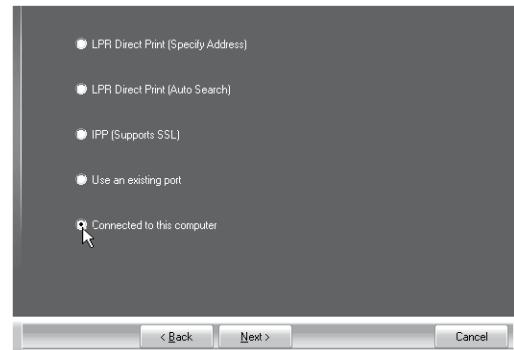
**4 When the port selection window appears, select the port that the PCL6 or Sharp Advanced Printing Language-c\* printer driver is using (USB001, etc.) and click the [Next] button.**
