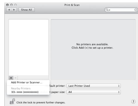
In Mac OS X v10.5 to 10.7, when the screen for adding a printer appears, click the + button.
