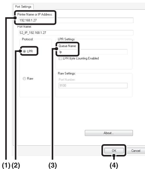
**(1) Enter the machine's IP address.**
