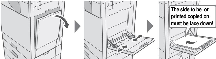
Load the paper in the horizontal orientation.
