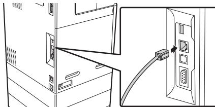
After connecting the machine to a network, be sure to configure the IP address and other network settings before installing the software. (The factory default setting for the IP address is to receive the IP address automatically when the machine is used in a DHCP environment.)
