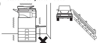
Vibration may cause failure.
