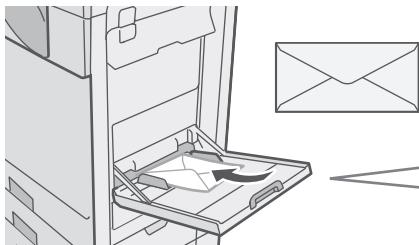
Only the address side of envelopes can be printed on. Place envelopes with the address side face down.
