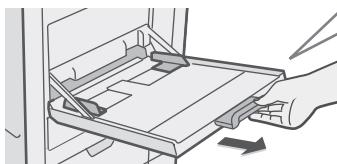
When loading paper larger than A4 or 8-1/2" x 11", pull out the tray extension.
