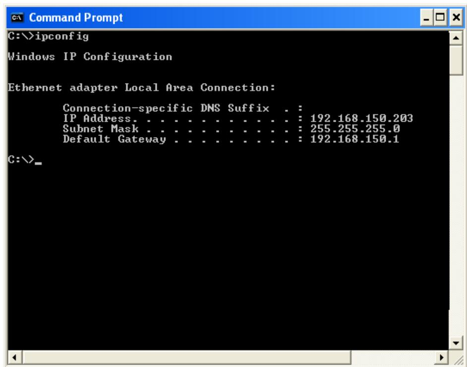
The screenshot shows a Command Prompt window with the title "Command Prompt". The window displays the output of the "ipconfig" command. The output shows the following details for the "Ethernet adapter Local Area Connection":
