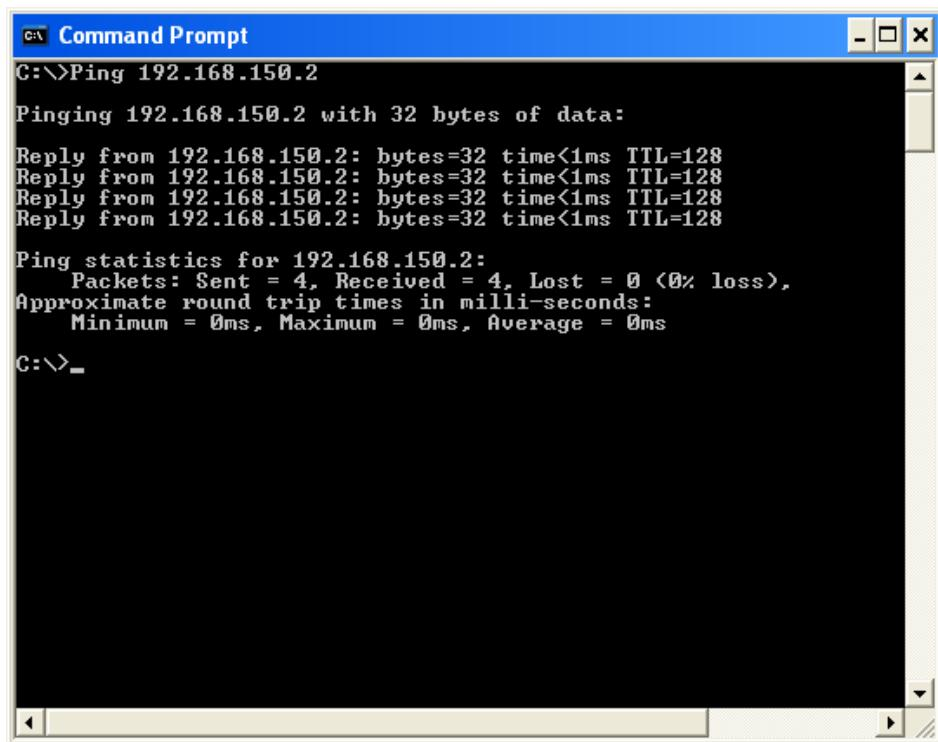
The screenshot shows a Windows Command Prompt window titled "Command Prompt". The command entered is "Ping 192.168.150.2". The output shows four replies from the target IP address, each with 32 bytes, a time less than 1ms, and a TTL of 128. It then provides ping statistics: 4 packets sent, 4 received, 0 lost (0% loss), and approximate round trip times of 0ms for minimum, maximum, and average.
