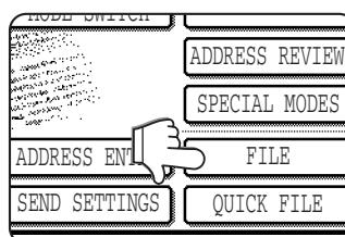
These keys are used to store the scanned image in the machine's hard disk. The stored image can be printed or transmitted again at a later time.
