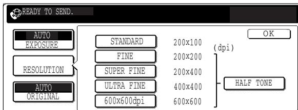
Five selections are available for the resolution. Touch the desired resolution key depending on the original to be scanned. For resolutions other than [STANDARD], the [HALF TONE] key can be selected.
