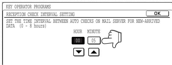
Touch the [HOUR] key and then set the hour by touching the and keys. Set the minute in the same way. When finished, touch the [OK] key.
