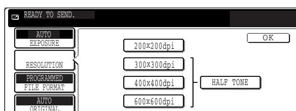
Four selections are available for the resolution. Touch the desired resolution key depending on the original to be scanned.
