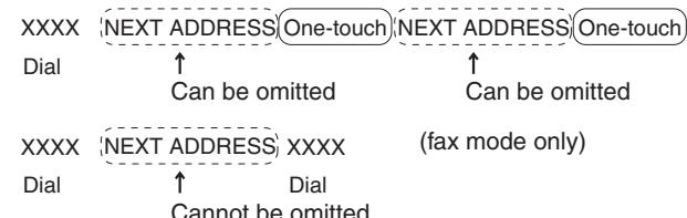
If the box is checked, it will no longer be possible to omit the [NEXT ADDRESS] key as shown in the above example. Even if the next destination to be entered is a one-touch key, the [NEXT ADDRESS] key must be touched before the one-touch key can be entered. If an operator attempts to enter the next destination without touching the [NEXT ADDRESS] key, an alarm will sound.
