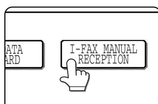
The machine connects to the mail server to check to see if new Internet-Fax data has been received. If new data has been received, this machine reads and prints it.
