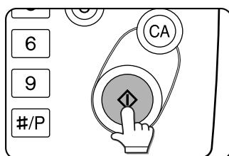
Scanning begins and the transmission job is stored. (The job is transmitted after previously stored transmission jobs have been completed.)
