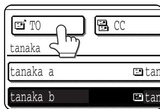
Normally touch the [TO] key. However, if you are performing a broadcast transmission and wish to "CC" or "BCC" the document to the entered address, touch the [CC] or [BCC] key.
