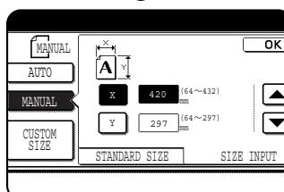
Touch the [X] key and use the  $\Delta$  or  $\nabla$  keys to set the length in the X direction, and then touch the [Y] key and do the same for the Y direction. The length can be within the range 64 to 432 mm (2-1/2" to 17") in the X direction and 64 to 297 mm (2-1/2" to 11-5/8") in the Y direction, set in increments of 1 mm (1/8").
