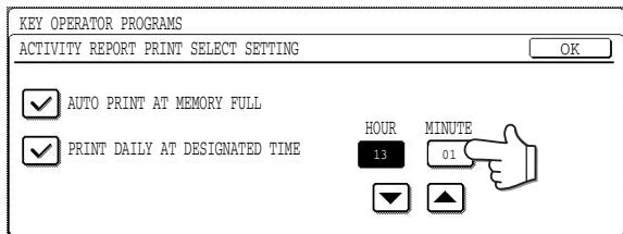
Touch the "HOUR" and "MINUTE" keys and then set the hour by touching the and keys. Set the minute in the same way. When finished, touch the [OK] key.
