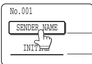
The "No." that automatically appears is the lowest number from 001 to 999 that has not yet been programmed. When [SENDER NAME] is touched, the letter-entry screen appears.
