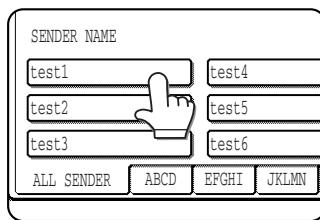
The selected sender name is highlighted. If you made a mistake, touch the correct key. The highlighting will move to the new key.
