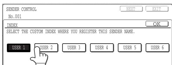
Select one of the six keys ([USER 1] through [USER 6]) to determine the location of the one-touch key when the GROUP index is displayed instead of the ABC index.
