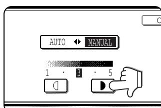
If you selected [MANUAL], touch the or key to adjust the exposure. (For darker contrast, touch the key. For lighter contrast, touch the key.)
