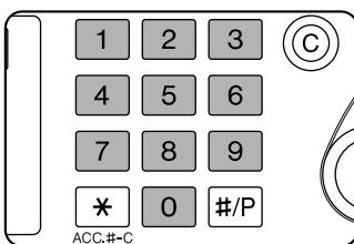
When a three-digit number is entered, the relevant address will be set as a destination address. Leading zeros (such as 00 in 001) can be omitted. In this case, when you touch the [NEXT ADDRESS] or
