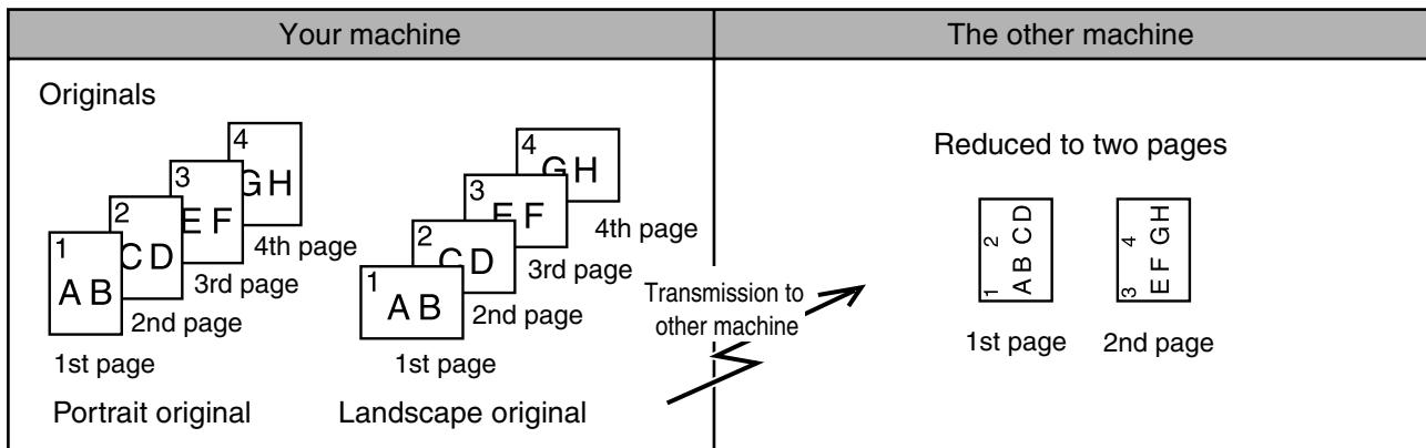
A3 and B4 (11" x 17", 8-1/2" x 14", and 8-1/2" x 13") sizes cannot be transmitted when using the 2 in 1 function. A4 (8-1/2" x 11") and smaller sizes can be used. There are restrictions on how the originals are placed. Both portrait and landscape oriented originals should be placed vertically as shown below.
