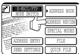
When the [ADDRESS REVIEW] key is touched, only the entered destinations are displayed. You can also display the CC and BCC destinations by touching the relevant keys.
