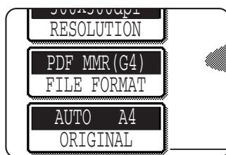
The original size is automatically detected. If you loaded a non-standard size document or wish to change the scanning size, touch the [ORIGINAL] key and set the document size. (Refer to [page 20](#).)
