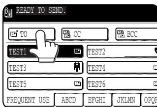
For Scan to E-mail, you can send the "CC" or "BCC" copies. Touch the desired destinations and then touch the [CC] key or [BCC] key. "BCC" can be set only if "ENABLE BCC" of the key operator program, "BCC Setting", is set. (page 56)
