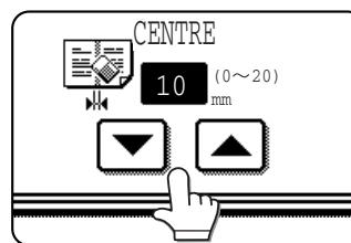
The erase width can be set from 0 mm (0") to 20 mm (1") in 1 mm (1/8") increments.
