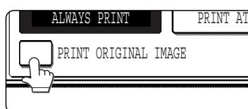
If the checkmark is displayed, a transaction report including the transmitted original will be printed.
