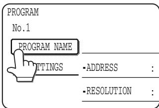
The "No." that automatically appears is the lowest number from 1 to 8 that has not yet been programmed. When the [PROGRAM NAME] key is touched, the letter-entry screen appears. Enter up to 18 characters for the name.
