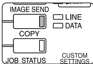
When the [IMAGE SEND] key light is on, the machine is in scanner mode. If the light is not on, press the [IMAGE SEND] key. Depending on the feature to be used, touch
