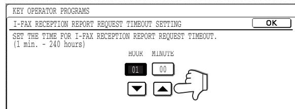
Touch the [HOUR] key and then set the hour by touching the and keys. Set the minute in the same way. When finished, touch the [OK] key.
