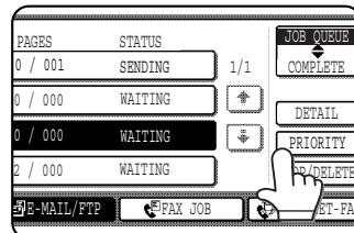
The selected job moves up to the next position after the job currently being executed. When the current job is completed, execution begins of the job selected in step 3.
