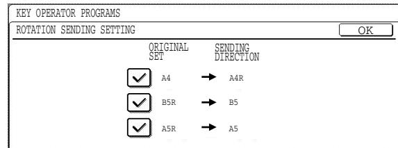
Rotation settings can be separately established for different document sizes. To turn off a rotation setting, touch the checkbox of the appropriate setting to remove the checkmark.
