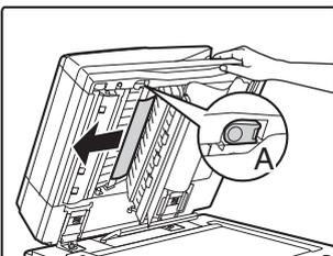
Press switch A to release the cover lock and remove the misfed original. After removing the original, be sure to attach the cover securely.
