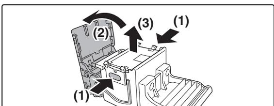
Press the sides from both directions (1) and open the cover in the direction of the arrow (2). Pull the empty staple case straight up and out of the cartridge (3).
