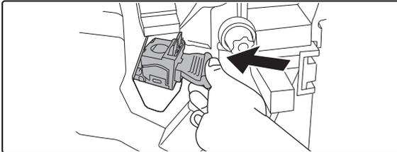
**Put the staple cartridge back into the stapler.**
