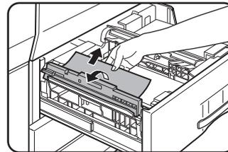
Lift the paper guide and remove the misfed paper. Be sure to replace the paper guide in its original position after removing the paper.
