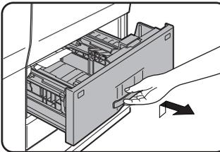
If misfed paper is not found in the previous step's illustration, pull out paper tray 1 - tray 2 and remove the misfed paper. Grasp the finger hold and gently open the unit. Pull the tray all the way out until it stops.
