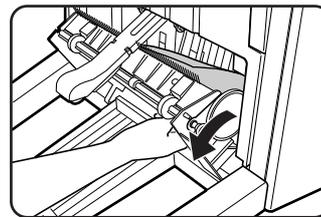
Open the exit cover of the saddle stitch unit and remove any misfed paper. Be careful not to tear the misfed paper during removal.
