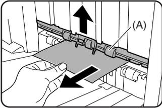
Lift (A) up in the direction of the arrow and remove any misfed paper. After removing the misfed paper, return (A) to its original position.
