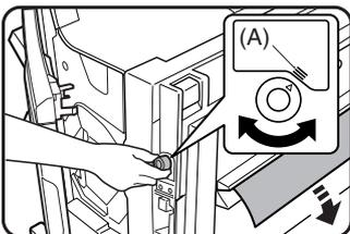
Rotate the green knob until the arrow is within the range (A) on the label, and remove the misfed paper. Be careful not to tear the misfed paper during removal.
