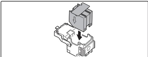
Insert a new staple case into the cartridge. Push the staple case all the way in until it clicks into place.
