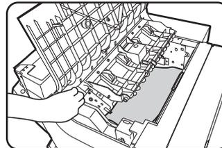
Lift knob (B) (see the previous step's illustration) and remove any misfed paper. Be careful not to tear the misfed paper during removal.
