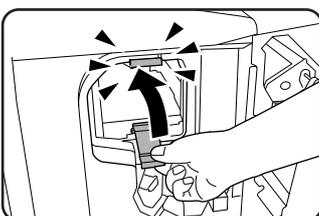
Lift the paper guide in the direction of the arrow. Push the paper guide until it clicks into place.
