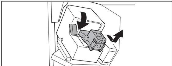
Lower the blue lever in the stapler and slide out the staple cartridge.
