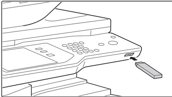
**Connect the USB memory to the USB connector (Type A) on the machine.**
