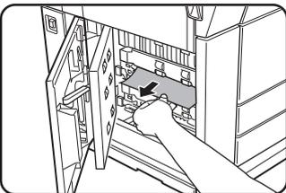
Remove the misfed paper. Be careful not to tear the misfed paper during removal.
