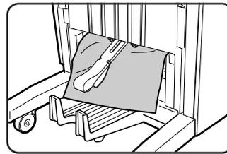
Remove any paper misfed on the exit side of the saddle stitch unit. Be careful not to tear the misfed paper during removal.
