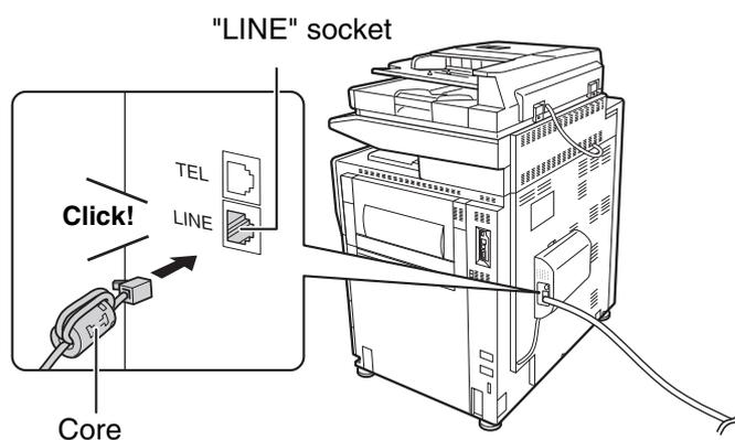
Insert the end of the cord with the core into the "LINE" socket.
