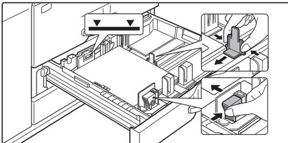
**Adjust the guide plates A and B by squeezing their lock levers and sliding them to the paper size to be loaded.**
