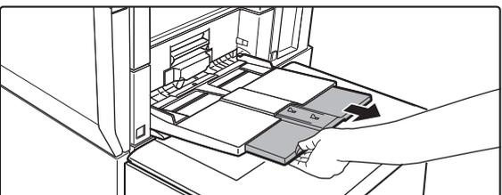
When loading A3, B4, A4R, 11" x 17", 8-1/2" x 14", 8-1/2" x 13" or 8-1/2" x 11"R paper, be sure to pull out the bypass tray extension. Pull the bypass tray extension all the way out. If the bypass tray extension is not pulled all the way out, the size of the loaded paper will not be correctly displayed.
