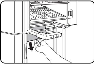
If a misfeed was not found in the above step, remove the misfed paper from under the paper guide. Be careful not to tear the misfed paper during removal.
