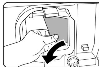
Remove any misfed paper. Be careful not to tear the misfed paper during removal.
