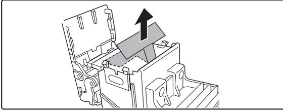
**Pull the seal that holds the staples straight out.**
