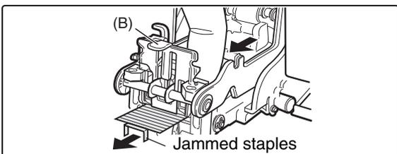
**Remove any jammed staples, and then return knob (B) to its original position.**
