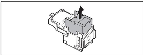
Pull the empty staple case straight up and out of the cartridge.
