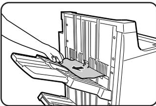
Remove any misfed paper from the paper exit area. Be careful not to tear the misfed paper during removal.
