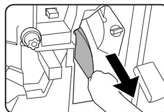
If there was no misfed paper in the previous step, remove any misfed paper. Be careful not to tear the misfed paper during removal.
