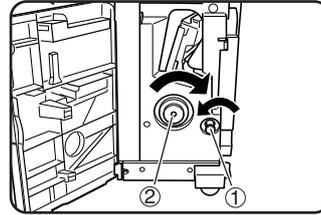
Turn the right-hand knob ① counter clockwise. Then, push the left-hand knob ② and turn it clockwise.
