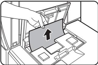
Open the top cover and remove the misfed paper. After removing the misfed paper, close the top cover.
