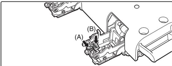
**While pushing down on lever (A), pull up knob (B).**
