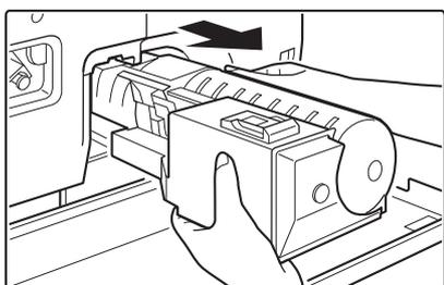
Hold the toner cartridge with both hands as shown in the illustration, and pull it out of the machine.
