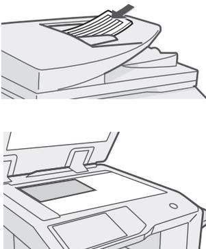
If the X dimension (width) of the document is less than 140 mm (5-1/2") or the Y dimension (height) is less than 131 mm (5-1/8"), place the original on the document glass. For a thin original, use "Slow Scan Mode".
