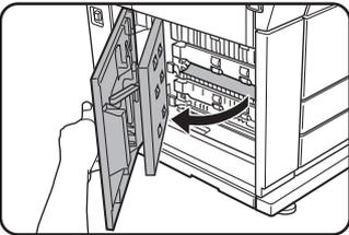
Open the lower cover on the left side of the machine. Grasp the finger hold and gently open the unit.
