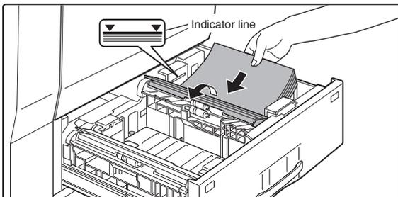
\*1 The paper stack must not be higher than the indicator line.
