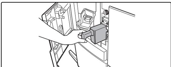
Holding the black handle, slide out the case containing the paper bits, and dispose of them properly.
