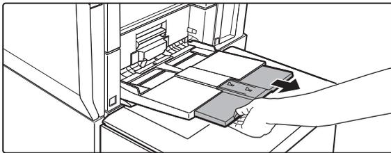
When loading paper larger than A4R or 8-1/2" x 11"R, be sure to pull out the bypass tray extension. Pull the bypass tray extension all the way out. If the bypass tray extension is not pulled all the way out, the size of the loaded paper will not be correctly displayed.
