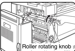
Turn roller rotating knob in the direction of the arrow to remove the misfed paper.
