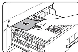
When using tray 2, bypass tray or large capacity tray, check the paper transfer unit inside the tray and remove any misfed paper.
