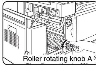
Remove the misfed paper. Turn roller rotating knob A in the direction of the arrow to remove the misfed paper.
