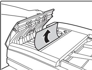
Open the document feeder cover and remove the misfed originals.
