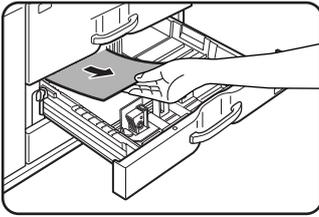
If misfed paper is not found in the previous step's illustration, pull out paper tray 3 and remove the misfed paper. Pull the tray all the way out until it stops. Check the paper transfer unit inside the tray. Be careful not to tear the misfed paper during removal.
