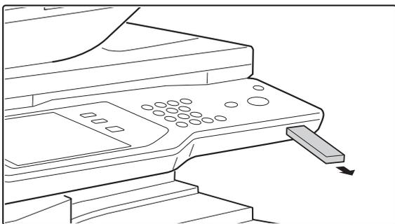
Remove the USB memory device from the machine.
