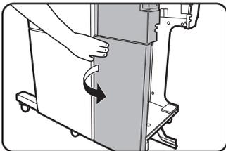
Open the front cover of the inserter (only when an inserter is installed).
