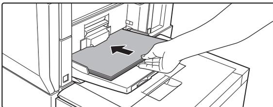
**Insert the paper along the bypass tray guides all the way into the bypass tray until it stops.**
