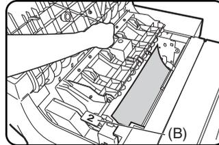
Lift knob (A) (see the previous step's illustration), then remove any misfed paper. Be careful not to tear the misfed paper during removal.
