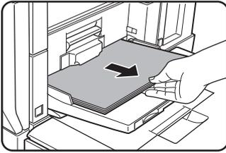
Remove the misfed paper from the bypass tray. Be careful not to tear the misfed paper during removal.
