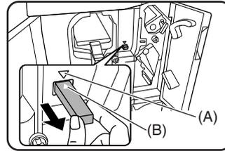
Pull out the green knob in the direction of the arrow. Align the triangle marks on (A) and (B), and remove any misfed paper. Be careful not to tear the misfed paper during removal.
