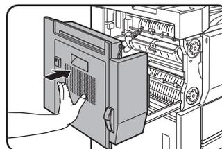
Gently close the duplex unit. After closing the duplex unit, confirm that the misfeed message has been cleared and the normal display appears.
