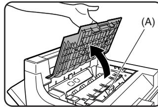
Open the upper cover of the finisher/saddle stitch finisher. When an inserter is installed, lift the tray of the inserter.
