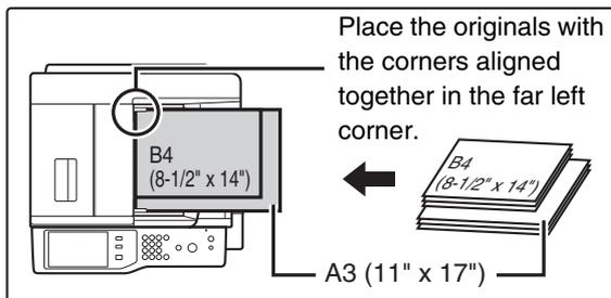
Place the originals with the corners aligned together in the far left corner.
